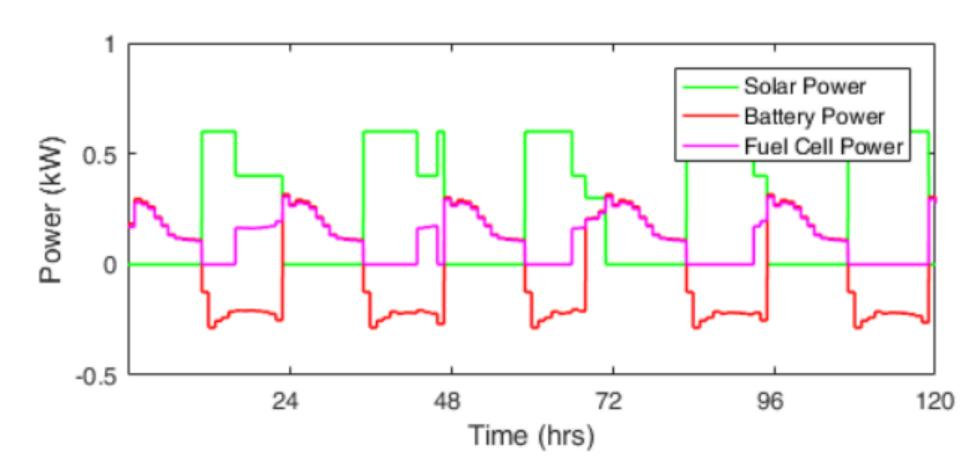
Simulated Solar, battery, and fuel cell contributions
